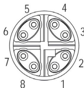
Ethernet connection pins, male (View onto the connector)
