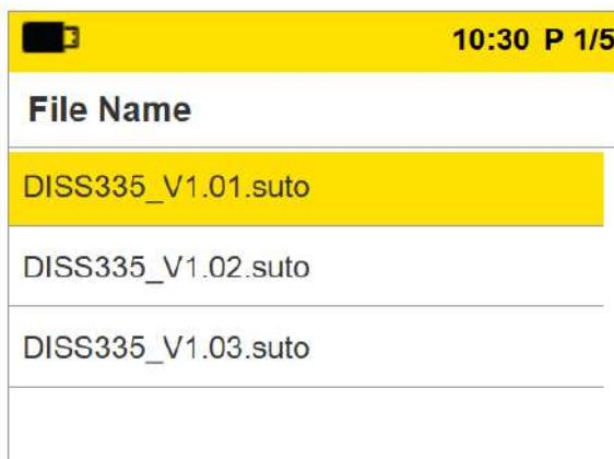
1. Insert the USB-C stick into the S335, then the firmware files with the .suto suffix are displayed automatically.
