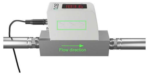
Due to the integrated flow conditioner, there are no additional straight pipe requirements for good measurement. However for best measurement, it is recommended 3-5 times inner diameter straight pipe at the inlet.
