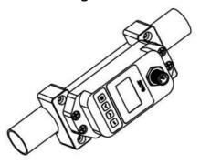
**Step 4**. Connect the cable to the M12 connector and then tighten them up.
