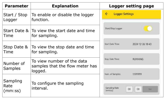
**Note**: When logger is started, it is not allowed to change any settings on either the device GUI or the S4C-FS app. If you try to change settings during logger running, the message "settings not allowed be change while logger is running" is displayed.
